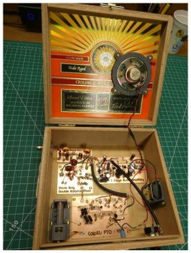
I was not satisfied with the "bare board" look, and so, I made a few "improvements." I found a cigar box of the proper size to hold all the boards and cut a thin piece of plywood to fit within the box.
