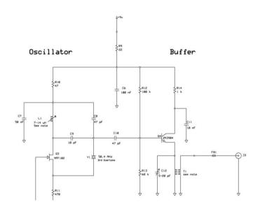
Note the little open circles where junction dots would normally be drawn (for example, at the intersection of Y1, Q3 and R11) and the occasional open circle where no junction would be (such as between T1 and FB1). These symbols represent the pads. Armed with that information, laying out the circuit becomes easy:
