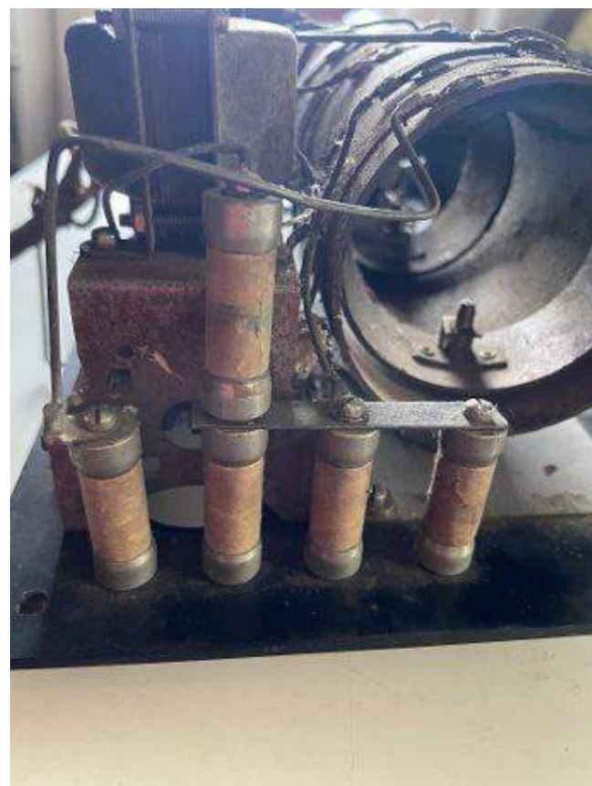
Capacitor Bank and Grid Leak
