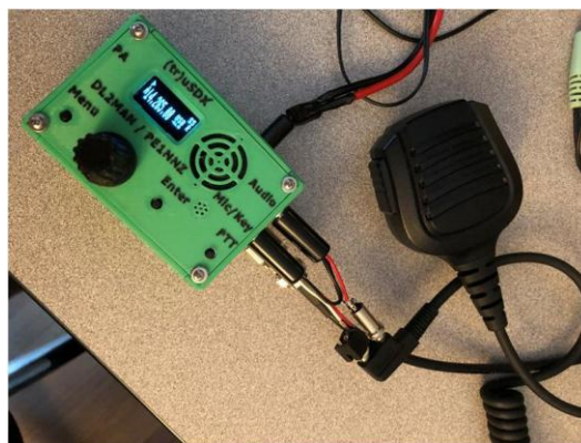
Figure 6 - External Speaker/Mic Wired Up
