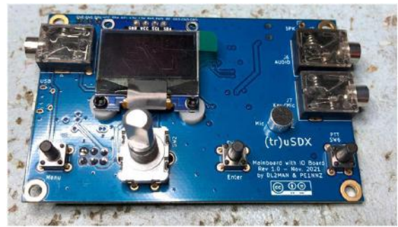
Figure 2 - Completed Main Board
