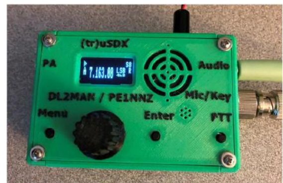
Figure 4 - Fully Assembled tr(uSDX) Mounted in the Case
