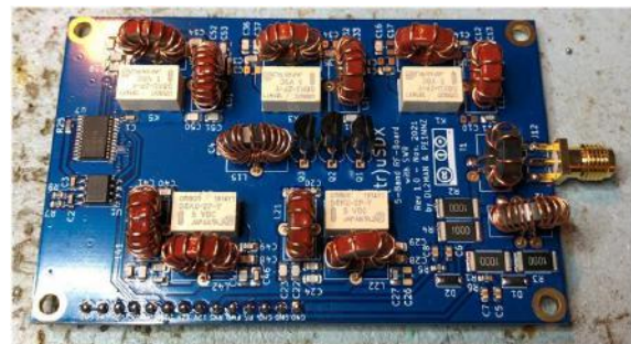
Figure 3 - Completed RF Board
