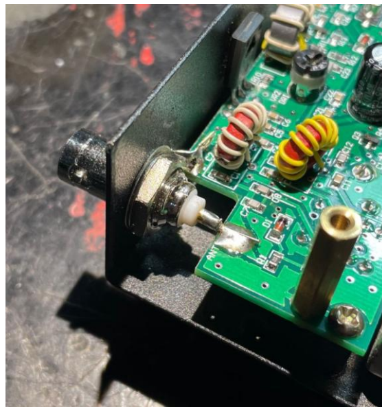
A Short Piece of Wire Makes the BNC Connector More Secure
