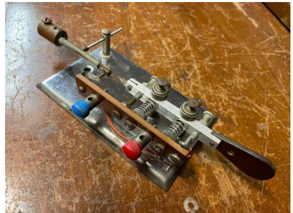
Overall Shot Showing Terminals and Dot Damper
