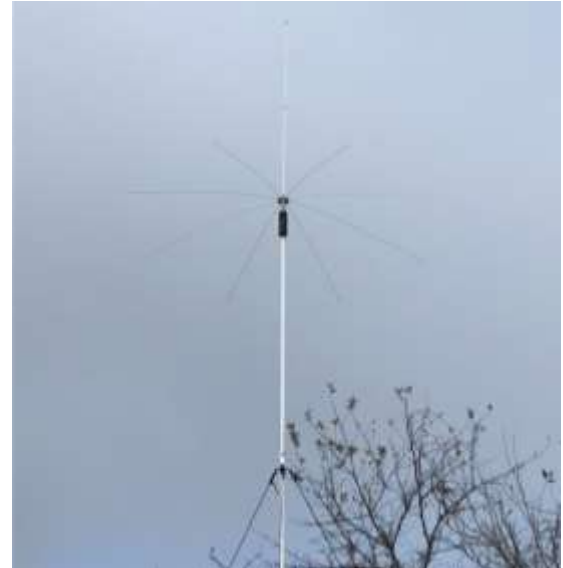
Figure 2 - Top of MA-160V Showing Loading Coil and Capacitance Hat
