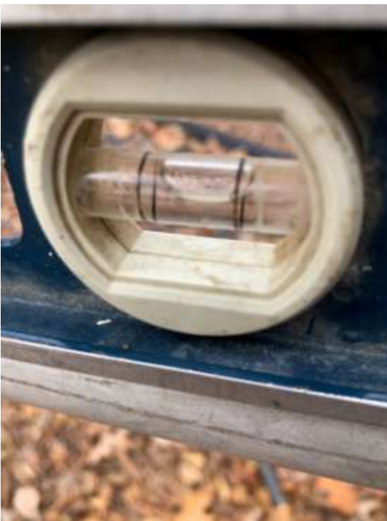
Figure 5: The Other Side of the Reflector. Note that the bubble is "off" an equal amount in the opposite direction from the previous photo when the element is aligned.
