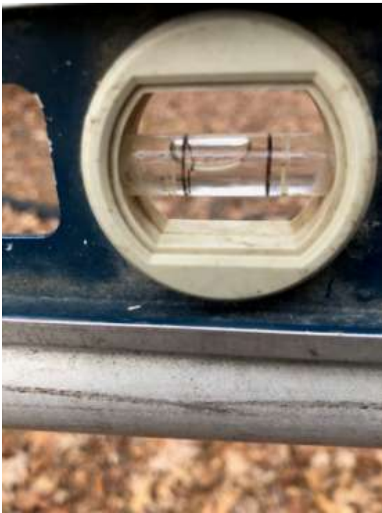
Figure 4: One Side of the Reflector. Note Position of Bubble due to Element Sag.
