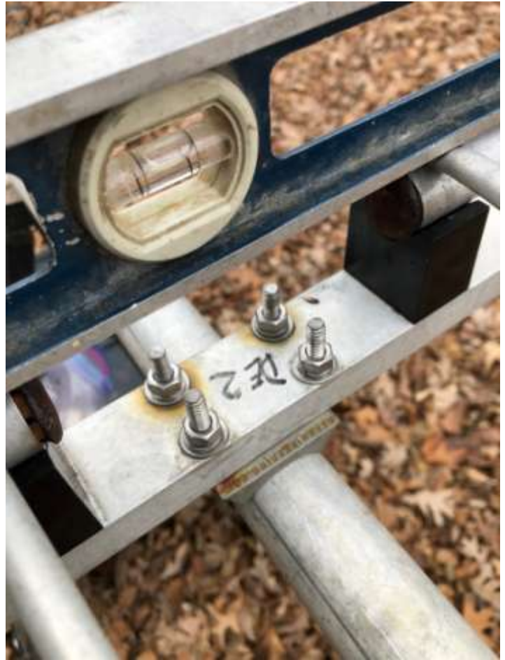
Figure 3: The Driven Elements have Reinforcements to keep their centers straight. Level them as shown here, across the center.
