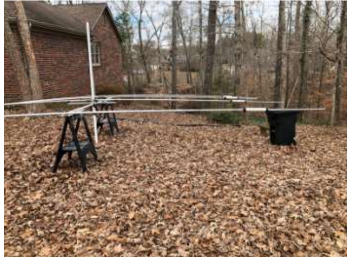
Figure 6: All Done! This antenna is probably 20 years old (I bought it used and upgraded the hardware.) Some elements sag slightly differently than others. This is about as aligned as you're going to get.
